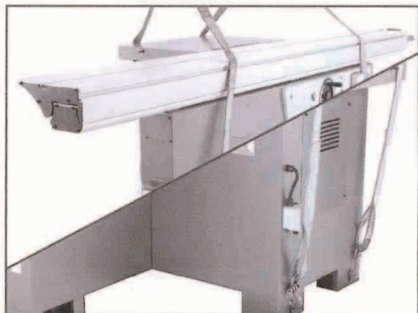
Figure 17. Lifting the saw base unit.
