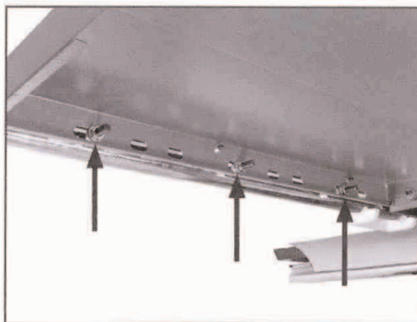
Figure 31. Rip fence rail adjustment nuts.
