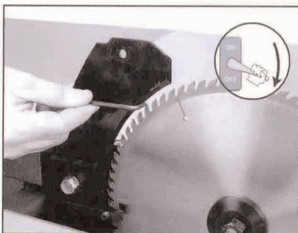
Figure 34. Adjusting the riving knife.
