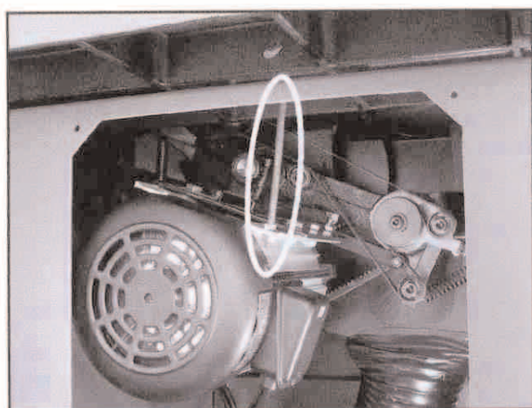
Figure 23. Motor support shipping bolt.
